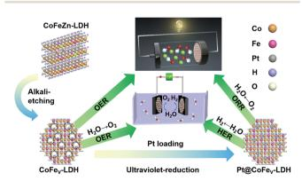
$\begin{tabular}{ll} Scheme 1 & Schematic illustration of the synthesis process for multifunctional $$Pt@CoFe_V-LDH.$ \end{tabular}$
