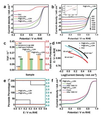
Fig. 5 (a) LSV curves of Pt/C, CoFe-LDH and Pt@CoFe $_V$ -LDH. (b) LSV curves of Pt@CoFe $_{1/3V}$ -LDH at various rotation speeds (inset: K-L plots for Pt@CoFe $_{1/3V}$ -LDH at 0.2 V vs. RHE). (c) Turnover frequency (TOF) and half-wave potential of Pt/C and Pt@CoFe $_V$ -LDH. (d) Tafel plots. (e) Peroxide percentage, electron transfer number and (f) LSV curves before and after 1000 CVs of Pt@CoFe $_V$ -LDH.
