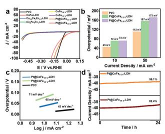
Fig. 4 (a) LSV curves of Pt/C, CoFe-LDH, CoFeZn-LDH, CoFe $_V$ -LDH and Pt@CoFe $_V$ -LDH for catalyzing the HER in 1.0 M KOH. (b) Histogram of the overpotentials of the Pt/C and synthesized nanomaterials to drive 10 mA cm $^{-2}$  and 50 mA cm $^{-2}$ . (c) Tafel slopes of Pt/C and Pt@CoFe $_V$ -LDH. (d) Long-term stability measurement of the Pt@CoFe $_V$ -LDH for over 24 h.
