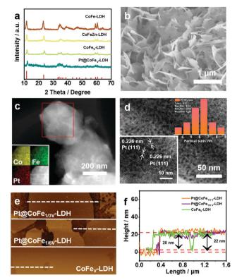
Fig. 1 (a) XRD patterns of CoFe-LDH, CoFeZn-LDH, CoFe $_V$ -LDH and Pt $_Q$ CoFe $_V$ -LDH. (b) FESEM image of the Pt $_Q$ CoFe $_V$ -LDH nanosheet. (c) TEM and EDS mapping images, (d) HRTEM of Pt $_Q$ CoFe $_V$ -LDH (inset: lattice space and size distribution of Pt NPs). (e and f) AFM images and curves of CoFe $_V$ -LDH and Pt $_Q$ CoFe $_V$ -LDH.
