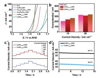
Fig. 3 (a) LSV curves of Ir/C, CoFe-LDH, CoFeZn-LDH and CoFe<sub>V</sub>-LDH for catalyzing the OER. (b) Histogram of the overpotentials of the Ir/C and CoFe<sub>V</sub>-LDH to drive 10 mA cm<sup>-2</sup> and 50 mA cm<sup>-2</sup>. (c) Multistep chronoamperometric curves of CoFe<sub>V</sub>-LDH at different applied potentials. (d) Long-term stability measurement of the CoFe<sub>V</sub>-LDH for over 18 h.
