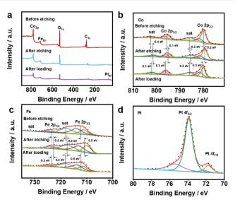
Fig. 2 XPS spectra of (a) the full, (b) Co 2p and (c) Fe 2p within CoFe<sub>V</sub>-LDH and Pt@CoFe<sub>V</sub>-LDH. (d) XPS spectra of Pt within Pt@CoFe<sub>V</sub>-LDH.
