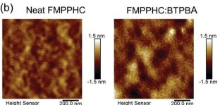
Fig. 2 (a) UV-Vis absorption and PL spectra in neat solid films of **FMPPHC** and BTPBA, and PL spectra in doping solid films of **FMPPHC** (host):BTPBA (dopant) with the doping concentration of 8 wt%. Inset: Molecular structure of BTPBA. (b) AFM topographical images of the solution-processed films of neat **FMPPHC** and **FMPPHC** doped with 15 wt% BTPBA.
