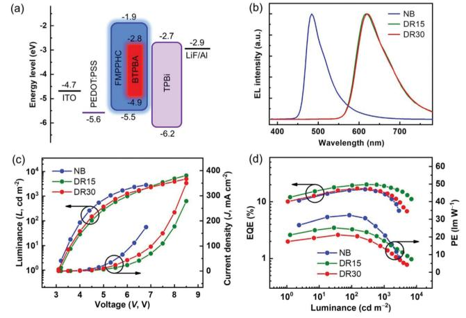
Fig. 3 (a) Proposed energy diagram of the materials used in OLEDs. (b) Normalized EL spectra of devices NB, DR15 and DR30 at the luminance of  $1000 \text{ cd m}^{-2}$ . Current density-voltage-luminance (J-V-L) curves (c) and power efficiency (PE)-luminance (L)-external quantum efficiency (EQE) curves (d) of devices NB, DR15 and DR30.
