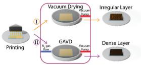
Fig. 1 Conventional vacuum drying leads to inhomogeneous perovskite crystallization and irregular thin films (I). By controlling the refilling of the chamber with N2-gas flow, so-called gas flow-assisted vacuum drying (GAVD), optical dense and pinhole-free perovskite layers (II) are achieved.
