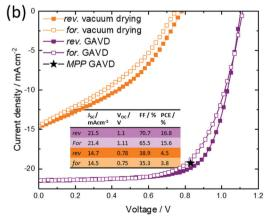
Fig. 4 (a) Solar cell architecture on p-i-n architecture. The Perovskite layer is inkjet-printed with the GAVD process. (b) Current density-voltage characteristics and of inkjet-printed perovskite solar cells on SAM using vacuum drying and GAVD method. Value for mpp-tracking (16%) is the average over 300 s of tracking the power output.
