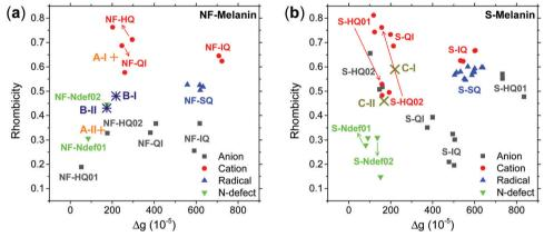
Fig. 5 The plot of the rhombicity as a function of g-value anisotropy for the different (a) NF-melanin and (b) S-melanin radical species. The theoretical radicals are represented by the square, circle and triangle symbols; the crosses are each of the experimental radicals. A purely isotropic signal would have  $\Delta q = 0$  and a completely axial symmetry signal would be obtained with rhombicity equal to 1.0 or 0.0.
