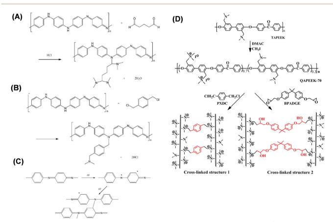
Fig. 6 Cross-linking PANI with (A) glutaraldehyde (GA), (B)  $\alpha, \alpha'$ -dichloro-p-xylene (DCX), and (c) thermal treatment. Copyright 2009, Elsevier. (D) Cross-linking TAPEEK using methyl iodide followed by PXDC (DCX) or BPADGE (Bisphenol A diglycidyl ether). 172 Copyright 2016, Elsevier.
