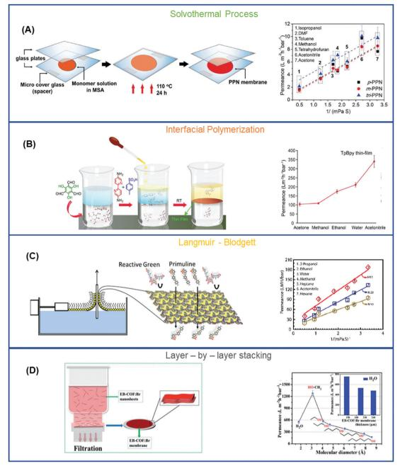
Fig. 10 Schematic representation for the preparation and performance of COFs prepared by using (A) SVT, <sup>74</sup> (B) IP, <sup>216</sup> (D) LB<sup>219</sup> and (D) LBL<sup>221</sup> methods. Copyright 2018 and 2020, The Royal Society of Chemistry. Copyright 2017 and 2018, American Chemical Society.
