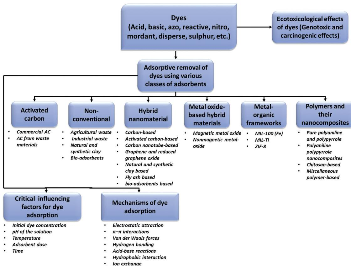
Fig. 4 Flow chart showing the classes of dye molecules, their ecotoxic effects, removal using different classes of adsorbents together with their sub-categories, critical influencing factors, and probable adsorption mechanisms.
