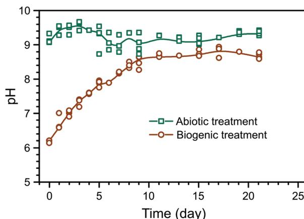
Fig. 1 Summary of pH evolution during the abiotic and biogenic treatment of the cement blocks; the coloured lines represent a B-spline through the median values of parallel experiments and are intended as a guide to the eye only.
