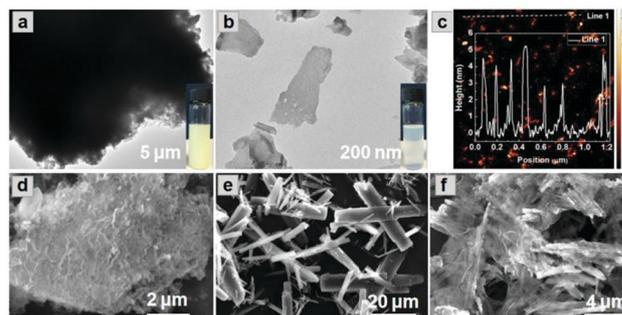
**Fig. 1** TEM images of (a) bulk  $g-C_3N_4$  and (b) CNNS exfoliated using  $scCO_2$ /CTAB. (c) AFM image of CNNS, inset: height of the CNNS as determined by AFM; SEM images of (d) bulk  $g-C_3N_4$ , (e) MFM-300(Fe), and (f) CNNS/MFM-300(Fe) composite. The composites shown here all have a  $g-C_3N_4$  : MOF wt : wt ratio of 7 : 3.
