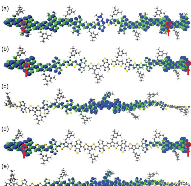
Fig. 3 The ground-state geometry and pictorial representations of spin density distribution for the (a) CPDT-TQ<sup>16</sup>, (b) CPDT-BBT, (c) CPDT-iso-BBT, (d) CPDS-BBT, and (e) CPDS-iso-BBT (N = 8) polymers in their S = 1 states. The blue and green surfaces represent positive and negative contributions of the spin density at an isovalue = 0.0002 a.u. The most probable locations for the unpaired electrons with largest atomic spin density are highlighted in open circles.
