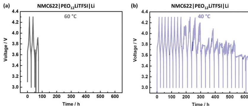
Fig. 1 Charge/discharge cycling of NMC622||Li cells with PEO-based SPE within a voltage range of 4.3 – 3.0 V and a specific current of 15 mA g<sup>-1</sup> ( $\approx 0.1C$ ) at (a) 60 °C and (b) 40 °C. The noisy voltage response during charge points to short circuits, whereby the onset of this failure tends to postpone at 40 °C.
