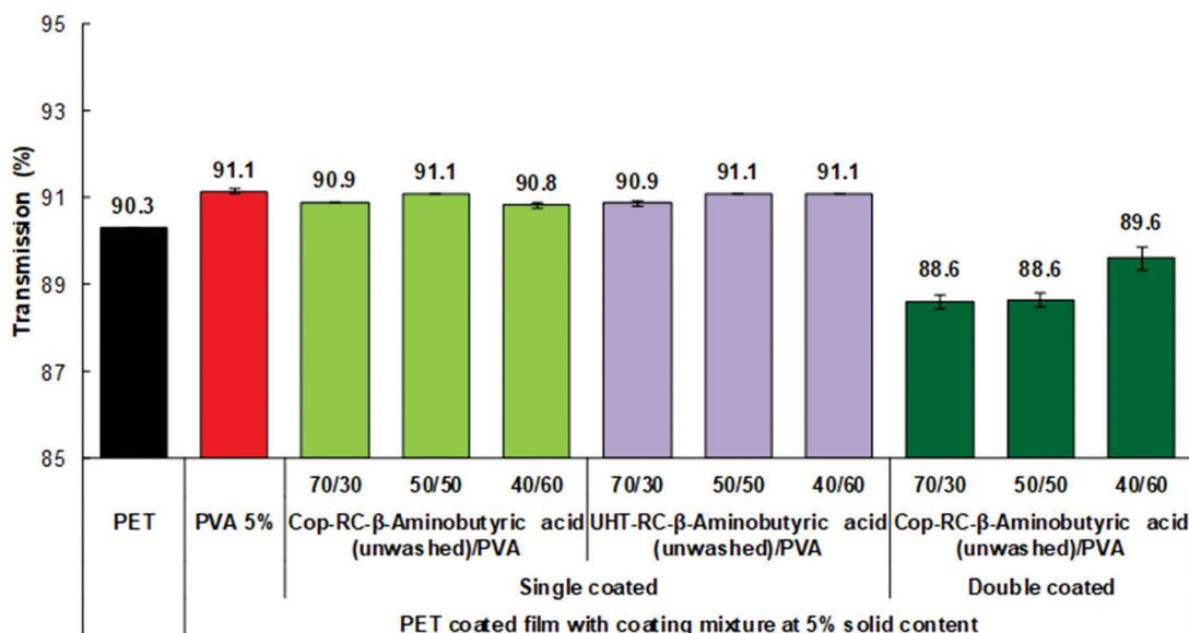
Fig. 4 Optical transmission of the coated films with Cop-RC- $\beta$  aminobutyric acid at different ratios with a 5 wt% solid content.
