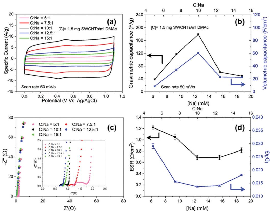
Fig. 2 Half-cell electrochemical performance, in 1 M  $\text{H}_2\text{SO}_4$ , of nanotubide buckypapers prepared from solutions at a given sodium concentration, or equivalent C : Na ratio: (a) CV curves at  $50 \text{ mV s}^{-1}$ ; (b) gravimetric and volumetric capacitance of (a) normalised to the mass and volume of active electrode; (c) Nyquist plots and (d) ESR and the  $I_D$  to  $I_G$  ratio derived from Raman spectra.
