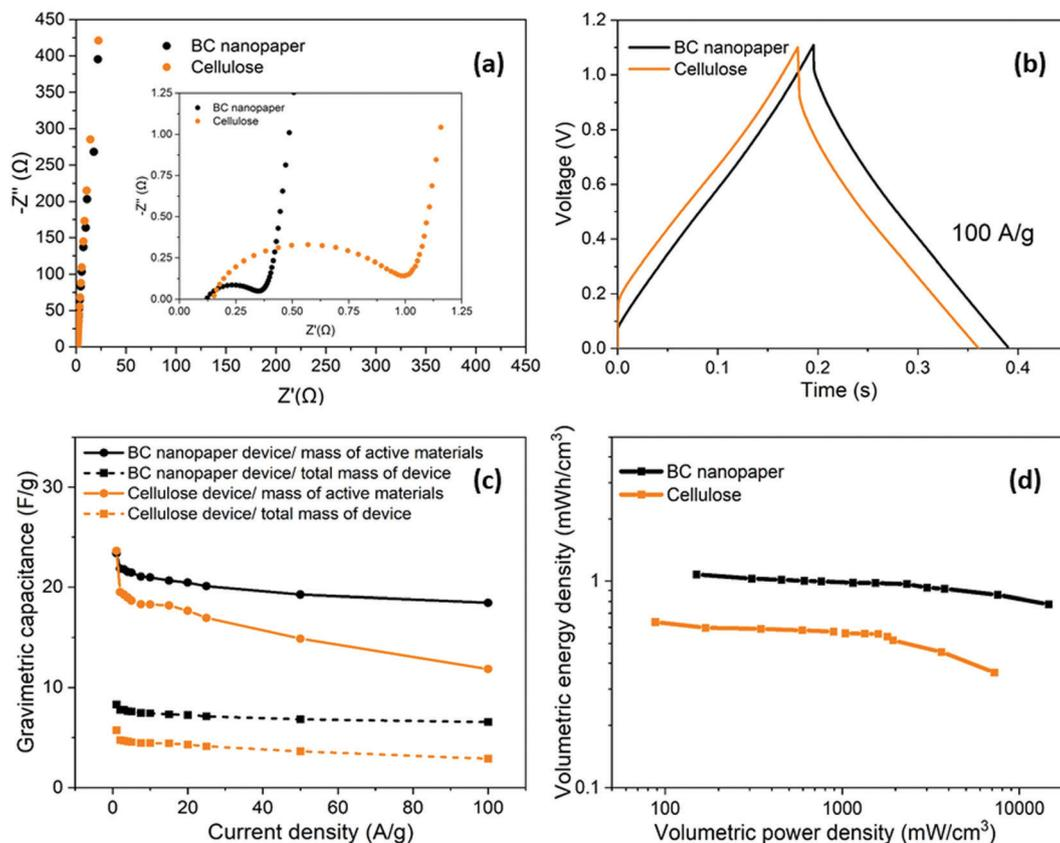
Fig. 4 Full-cell electrochemical performance of aqueous symmetric supercapacitors using nanotubide buckypaper electrodes sandwiched with BC nanopaper (black) and cellulose (orange) as separators: (a) Nyquist plots and (b) GCD curves at 100 A  $\text{g}^{-1}$ , (c) the calculated gravimetric capacitance normalised by both active material (straight line) and total mass of device (dash line) and (d) volumetric Ragone plots normalised by total mass of device.
