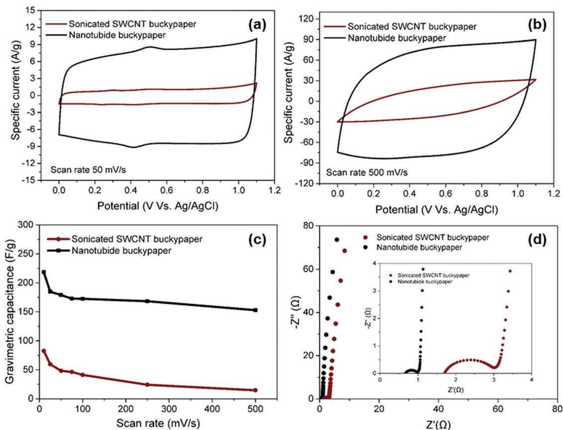
Fig. 3 Half-cell electrochemical performance, in 1 M H<sub>2</sub>SO<sub>4</sub>, comparing optimised nanotubide buckypaper to a conventionally processed control: (a) CV curves at 50 mV s<sup>-1</sup>, (b) CV curves at 500 mV s<sup>-1</sup>, (c) gravimetric capacitance as a function of scan rate normalised by mass of active electrode and (d) Nyquist plots.
