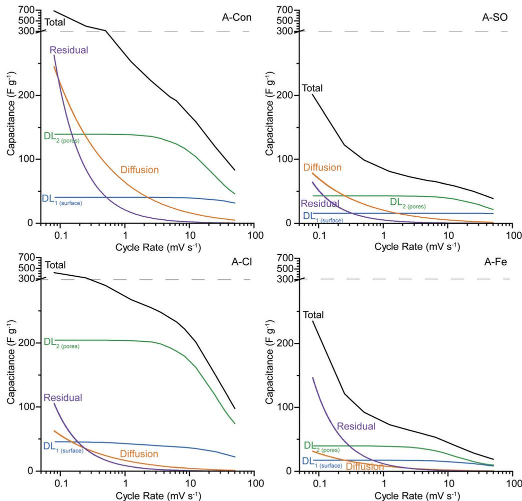
Fig. 8 SPECS analysis for (a) A-Con, (b) A-SO, (c) A-Cl, and (d) A-Fe. The y-axis has been split at  $300 \text{ F g}^{-1}$  (dashed line) to allow easier comparison between samples. A-PO was not included as it was unstable under cycling.
