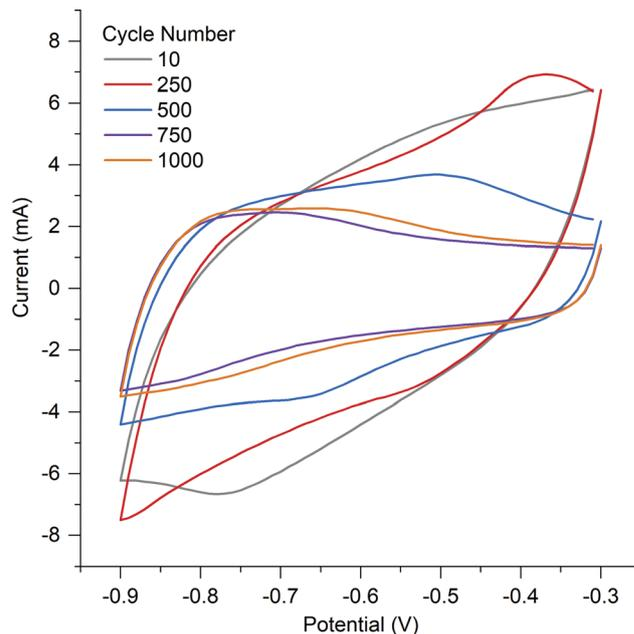
Fig. 6 Cyclic voltammetry of A-PO at different cycles.
