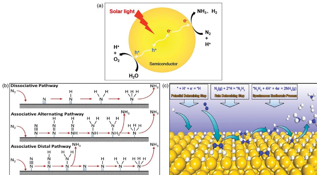
**Fig. 1** (a) Photocatalytic synthesis of  $\text{NH}_3$  in water. (b) The proposed mechanisms for photocatalytic  $\text{N}_2$  reduction consisting of the dissociative pathway, the associative alternating pathway, and the associative distal pathway. Reproduced from ref. 27 with permission from ACS Publication. (c) The proposed mechanism of surface-hydrogenation over noble metal doped photocatalysts for NRR. Reproduced from ref. 28 with permission from ACS Publication.
