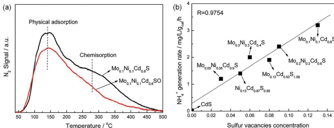
**Fig. 6** (a) The  $\text{N}_2$ -TPD of  $\text{Mo}_{0.1}\text{Ni}_{0.1}\text{Cd}_{0.8}\text{S}$  and  $\text{Mo}_{0.1}\text{Ni}_{0.1}\text{Cd}_{0.8}\text{SO}$ . (b) The relationship of  $\text{NH}_3$  yield over the obtained photocatalysts and the SV concentration. Reproduced from ref. 57 with permission from The Royal Society of Chemistry.
