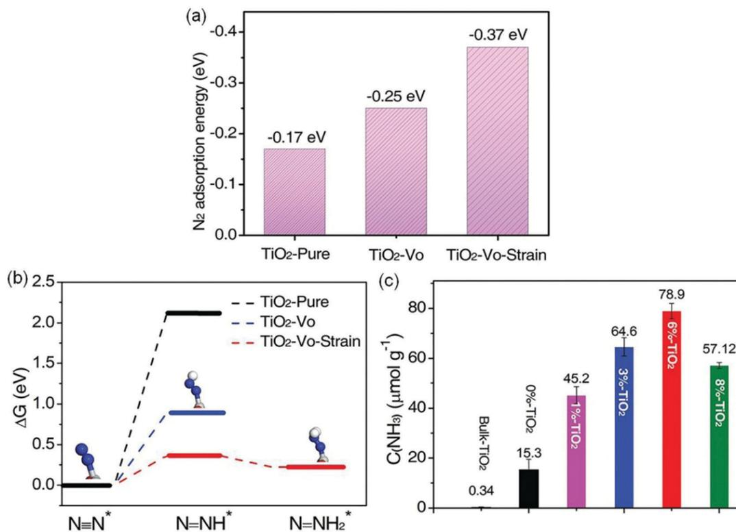
**Fig. 8** (a) The  $\text{N}_2$  adsorption energies by DFT calculations on different photocatalysts. (b) The calculated Gibbs free energy for  $\text{N}_2$  reduction on the (001) surface of different photocatalysts (H: white sphere, Ti: gray sphere, N: blue sphere, O: red sphere). (c) Yield of  $\text{NH}_3$  over various samples under UV-vis irradiation. Reproduced from ref. 68 with permission from Wiley-VCH.
