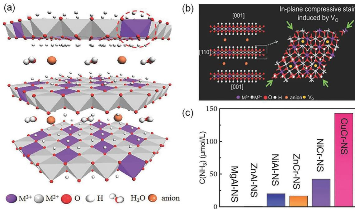
Fig. 4 (a) Schematic representation of the layered LDH structure with defective MO<sub>6</sub> octahedra. (b) Schematic of the in-plane biaxial compressive strain in CuCr-NS. (c) The yield of NH<sub>3</sub> over different LDH photocatalysts under visible-light illumination ( $\lambda > 400$  nm). Reproduced from ref. 34 with permission from Wiley-VCH.
