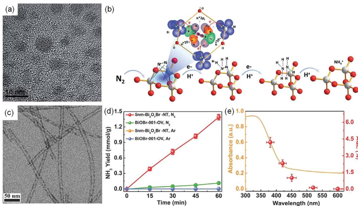
Fig. 10 (a) TEM image of BiO quantum dots. (b) Proposed mechanism for  $N_2$  photoreduction on BiO quantum dots. Reproduced from ref. 86 with permission from The Royal Society of Chemistry. (c) TEM image of  $Bi_5O_7Br$ -NT. (d) Yield of  $NH_3$  for  $Bi_5O_7Br$ -NT. (e) The wavelength-dependent AQE of  $Bi_5O_7Br$ -NT. Reproduced from ref. 87 with permission from Wiley-VCH.
