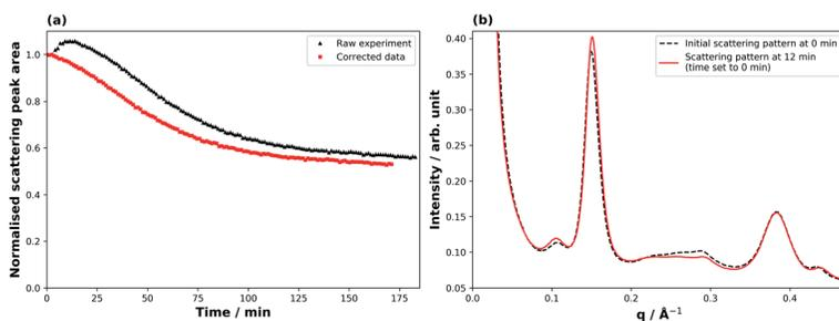
Fig. 2 Illustration of data correction (film thickness:  $73 \pm 2\text{ }\mu\text{m}$ ). (a) Scattering peak area vs. time exposed to ozone; both raw and corrected data are plotted. (b) SAXS patterns of the sample at the beginning of the experiment (black dashed line) and at the time (after 12 min) at which the peak scattering area was measured, which was defined as  $t = 0$  for the decay of the lamellar phase (red solid line).
