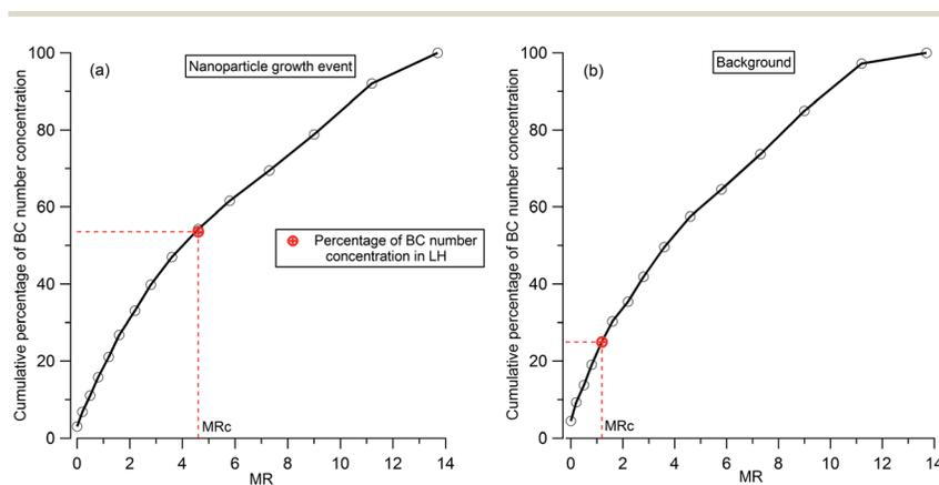
Fig. 5 Examples of the derivation of critical coating thickness (MR<sub>c</sub>) for 250 nm BC-containing particles: (a) high MR<sub>c</sub> condition as indicated by the red arrow in Fig. 4(d); (b) low MR<sub>c</sub> condition as indicated by the grey arrow in Fig. 4(d). The red circle represents the percentage number concentration of 250 nm BC-containing particles in LH.
