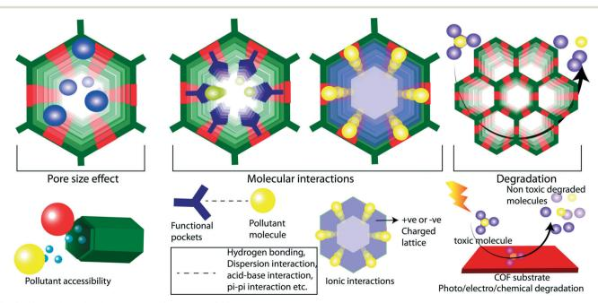
Fig. 4 Mechanism of pollutant removal/capture by COFs.
