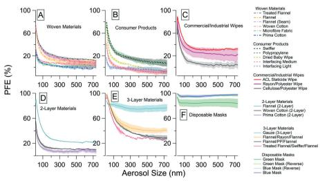
Fig. 3 PFE as a function of aerosol size for all tested materials and multi-layer combinations, grouped according to material class: (A) woven materials; (B) consumer products; (C) commercial/industrial wipes; (D) 2-layer materials; (E) 3-layer materials; and (F) disposable masks. Variability shown is one standard deviation of the mean for the three tests.
