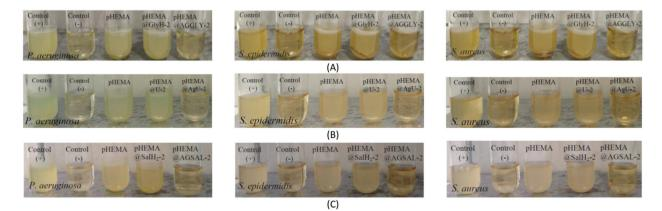
Fig. 5 Bacterial (P. aeruginosa, S. epidermidis and S. aureus) viability when they are incubated over pHEMA; A: pHEMA@GlyH-2 and pHEMA@AGGLY-2; B: pHEMA@U-2 and pHEMA@AGU-2 and C: pHEMA@SalH2-2 and pHEMA@AGSAL-2 under continuous stirring.
