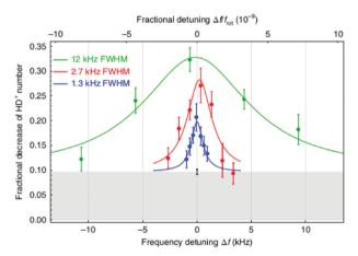
Fig. 18 (Top) Setup for sympathetic cooling and rotational spectroscopy of HD<sup>+</sup> (L-RC: rotational cooling laser, L-PD: photodissociation laser, L-C: Be<sup>+</sup> cooling laser). (bottom) Spectroscopy signal of two unresolved hyperfine components  $(N,F,m_F)=(1,3,\pm 3)\leftarrow (0,2,\pm 2)$  of the fundamental rotational transition of HD<sup>+</sup>. The different traces were recorded at different power levels. Figures reprinted from ref. 147 with permission of Springer Nature
