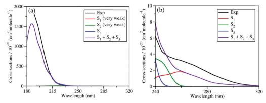
Fig. 2 Comparison of experimental and simulated UV absorption spectra of CH<sub>3</sub>ONO<sub>2</sub>: (a) from 180 nm to 320 nm; (b) from 240 nm to 320 nm. The theoretical spectra were simulated at XMS(4)-CASPT2(12,9)/def2-SVPD level. The experimental spectra in (a) and (b) were taken from previous works. 6,27 The intensities of absorption bands shown in (a) and (b) differ by several magnitudes.
