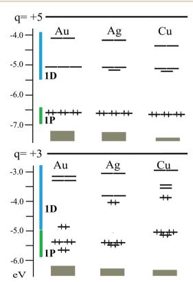
Fig. 2 Electronic structure for  $M_{13}(dppm)_6$  at +5 and +3 charge states. M = Au, Ag, and Cu 1P and 1D superatomic shells are denoted by green and
