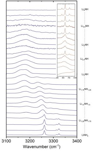
Fig. 5 The N-H stretching region of the Raman spectra of the Li-N-H samples, and inset, the low-energy region of the imide-nitride-hydride samples.
