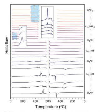
Fig. 6 Differential scanning calorimetry data for the Li-N-H samples. An endothermic event is a positive change in the heat flow. Inset are the highlighted regions for the melting of lithium amide and the phase transition of lithium imide
