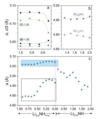
Fig. 4 Lattice parameters of (a) lithium amide (b) lithium nitride-hydride and (c)  $Fm\bar{3}m$  phases (and  $0.5 \times a$  for the  $Fd\bar{3}m$  Li<sub>2</sub>NH phase), with an inset plot of the highlighted amide-imide region. Error bars are smaller than the data points.
