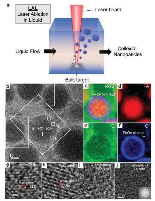
Fig. 3 Formation of amorphous Fe oxide NPs by laser ablation in an organic solvent. (a) Schematic illustration of laser ablation in liquid. (b-f) TEM image and the corresponding EDX mapping of a Fe@FeO $_x$  core-shell NP by fs-laser ablation in acetone. (g-j) HRTEM of the selected position of the NP in (a) showing different shell structures and an amorphous core. Reproduced with permission from ref. 147.
