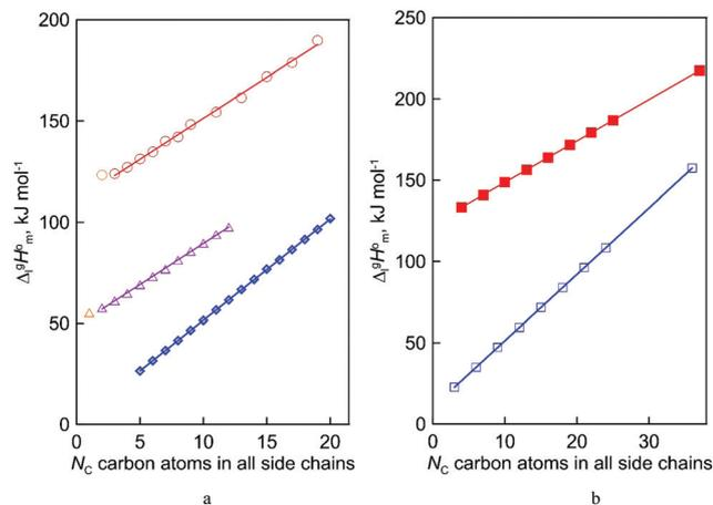
Fig. 2 Vaporization enthalpies' at 298 K (in  $\text{kJ mol}^{-1}$ ) chain-length dependences of molecular and ionic compounds: (a) alkanes (opened diamonds,  $\diamond$ ),<sup>12,13</sup> alkyl-imidazoles (opened triangles,  $\triangle$ )<sup>14</sup> and 1-methyl-3-alkyl-imidazolium based ILs (opened circles,  $\circ$ );<sup>10</sup> (b) trialkylamines<sup>15</sup> (opened squares,  $\square$ ) and tetraalkylammonium based ILs from this work (solid squares,  $\blacksquare$ ).
