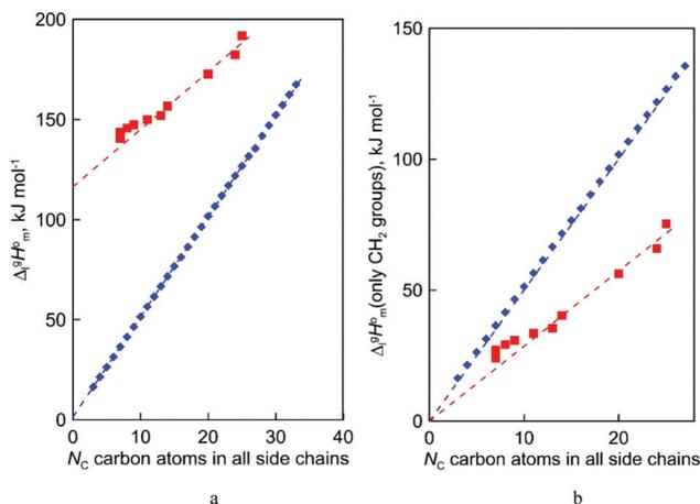
Fig. 5 (a) The chain length dependence of the vaporization enthalpies for  $n$ -alkanes,  $C_nH_{2n+2}$  (diamonds,  $\blacklozenge$ ); ammonium-based ILs with the  $[NTf_2]^-$  anion, (squares,  $\blacksquare$ ). Primary experimental data for correlations are given in Tables S11–S15 (ESI $^\dagger$ ). (b) The dispersion part of the vaporization enthalpy due to the alkyl chains.
