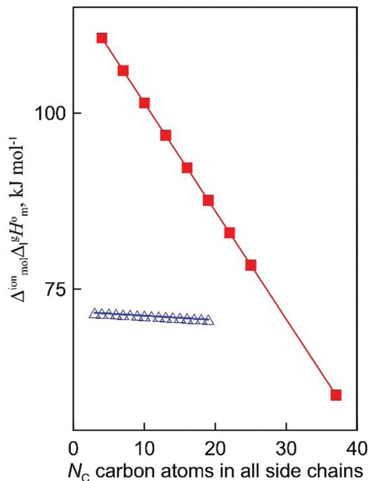
Fig. 3 Differences (in  $\text{kJ mol}^{-1}$ ) between the  $\Delta_1^g H_m^\circ$  (298.15 K)-values for the ionic and molecular compounds. 1-Methyl-3-alkyl-imidazolium based ILs<sup>10</sup> and alkyl-imidazoles<sup>14</sup> (opened triangles,  $\triangle$ ); tetraalkylammonium based ILs from this work and trialkylamines<sup>15</sup> (solid squares,  $\blacksquare$ ).
