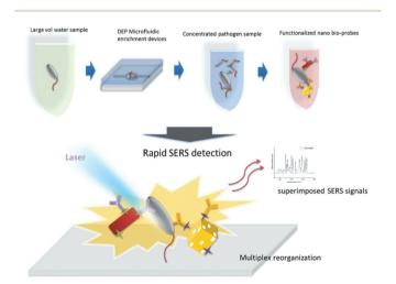
Fig. 2 Schematic describing the rapid enrichment step using a microfluidic device and detection step using a multiplex self-referencing SERS strategy. Three anisotropic SERS tags, designed to target different epitopes on E. coli O157:H7 cells, were employed to yield a dual SERS signal containing contributions from the target pathogen and nanotags that confirmed specific pathogen recognition. The image is reprinted from Wang et al., 65 Copyright (2017), with permission from BioMed
