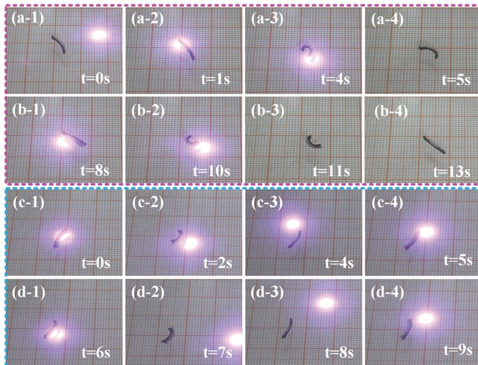
**Fig. 6** The 90° circulatory and the homodromous circulatory switching processes of NFC2 gradient intelligent hydrogels. (a-1)–(a-4) Switching 90° to left and (b-1)–(b-4) switching 90° to right with a power density of 6.32 W cm<sup>-2</sup>. (c-1)–(c-4) The first, and (d-1)–(d-4) the second switching process with a power density of 18.7 W cm<sup>-2</sup>.
