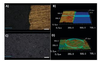
Fig. 2 Height mapping images and 3D views realized with a confocal laser microscope at a magnification of ×50 of WS<sub>2</sub>-COOH film at the cut edge (A and B) with the film on the left and the substrate on the right. Microscope images of the center of the film (C and D).
