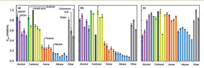
Fig. 5 Response of MOF-MSS array sensor membranes spray-coated with (a) ZIF-7, (b) ZIF-65-Zn, and (c) ZIF-71. Relative mean response magnitudes are calculated from three measurements for each gas; error bars represent two standard deviations. Colours correspond to those used in Fig. 2.
