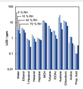
Fig. 3 Limit of detection (LOD) of a 2100 droplet nanoparticle ZIF-8-MSS sensor fabricated by inkjet deposition towards various analytes determined at 25 °C and humidity levels from 0% RH (light blue) to 70% RH (dark blue). MCH = methylcyclohexane; EtOAc = ethyl acetate; prop.acid = propionic acid.
