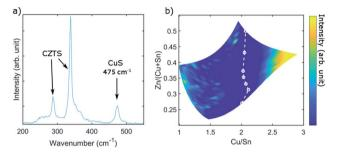
Fig. 2 (a) Raman spectrum (532 nm excitation) with CZTS Raman modes in the range 250-400 cm<sup>-1</sup>. CuS mode visible at 475 cm<sup>-1</sup>. (b) Integrated intensity in the region of the CuS peak against the cation composition from EDX. The phase boundary for CuS is marked with a white dashed line.
