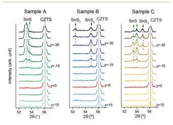
Fig. 4 XRD patterns of samples A, B and C in a  $2\theta$  range with expected SnS and SnS<sub>2</sub> reflections. y denotes the distance to the Cu/Sn = 2 line in mm.
