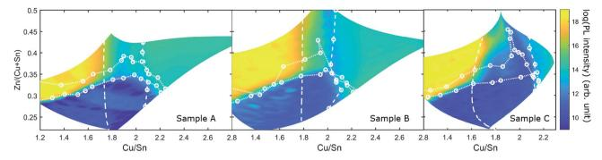
Fig. 9 Map of the logarithm of the integrated PL intensity of samples A, B and C. The secondary phase boundaries determined from Raman and XRD are shown as white dotted and dashed lines.
