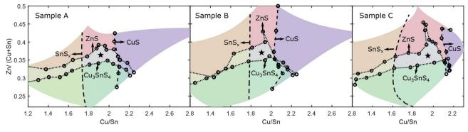
Fig. 5 Phase boundaries from Raman and XRD measurements for samples A, B and C. The regions with secondary phases are shaded in different colours. The CZTS single-phase region is denoted with a star.
