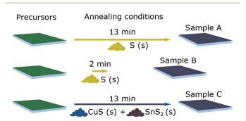
Fig. 1 Sample overview illustrating the different processing conditions during the annealing step in terms of annealing time and atmosphere. The annealing temperature is  $550\,^{\circ}$ C.
