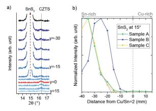
Fig. 3 (a) XRD patterns in regions with SnS<sub>2</sub> reflection at 15° for different positions parallel to the Cu/Sn = 2 line on sample B. y denotes the distance to the Cu/Sn = 2 line in mm. (b) Integrated intensity of the reflection at 15°. The dotted lines are guides to the eye for the interpolation to the phase boundary.
