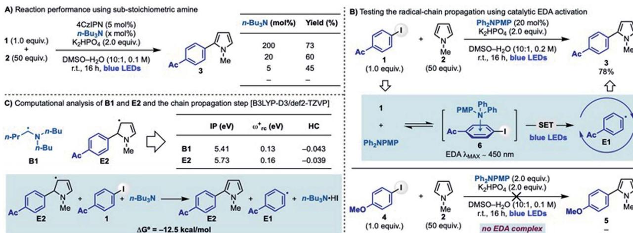
Scheme 3 (A) Impact of the *n*-Bu<sub>3</sub>N stoichiometry on the radical coupling between 1 and 2. (B) Radical couplings via EDA. (C) Computational studies on key properties of  $\alpha$ -aminoalkyl radical (B1) and extended aminoalkyl radical (E2) and the thermodynamic feasibility of the chain propagation step. PMP = *p*-OMe-C<sub>6</sub>H<sub>4</sub>.
