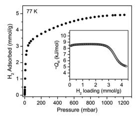
Fig. 2 Hydrogen adsorption isotherm for 1, measured at 77 K. Inset: loading-dependent isosteric heat of adsorption ( $Q_{st}$ ) for  $H_2$  in 1.
