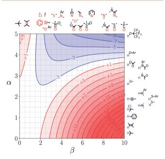
Fig. 6 FGIP for the interaction of two solutes in 1,1,1,3,3,3-hexafluoro-2-propanol at 298 K ( $\Delta\Delta G_{FGI}$  in kJ mol<sup>-1</sup>). The solute-solute interactions in the blue region, and unfavourable in the red region.
