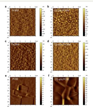
Fig. 5 AFM height images of (a) PCBM, (b) (S)-pSi/PCBM, (c) ThCBM, (d) (S)-pSi/ThCBM, (e) PCBE, and (f) (S)-pSi/PCBE films after annealing at 150 °C for 30 min.
