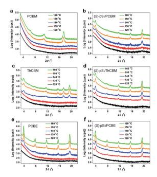
Fig. 4 Out-of-plane XRD patterns of pure (a) PCBM, (c) ThCBM, and (e) PCBE films annealed at different temperatures. The films were prepared by spin-coating the fullerene derivative solutions (10 mg mL $^{-1}$ ). Out-of-plane patterns of (b) (S)-pSi/PCBM, (d) (S)-pSi/ThCBM, and (f) (S)-pSi/PCBE annealed at different temperatures. The films were prepared by spin-coating the (S)-pSi (1.5 mg mL $^{-1}$ ) and fullerene derivative (10 mg mL $^{-1}$ ) blend solutions.
