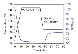
Fig. 2 Overview of TGA adsorption kinetics assay. The diamine-appended metal-organic framework sample is activated within a thermogravimetric analyzer under flowing  $N_2$  to remove solvent molecules and non-metal-bound diamines from the pores. The sample is then cooled under  $N_2$  to the temperature of interest, the gas flow is switched to a  $CO_2$ -containing stream, and  $CO_2$  adsorption is monitored as a function of time.
