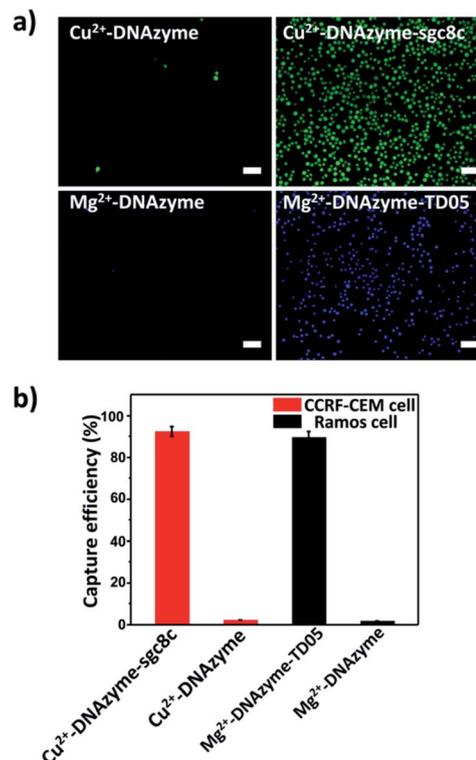
Fig. 3 (a) Fluorescence images: CTC capture capability study of our proposed platform using different capture elements on the substrate; scale bars: 50  $\mu$ m; (b) capture efficiencies of CTCs by different capture elements.
