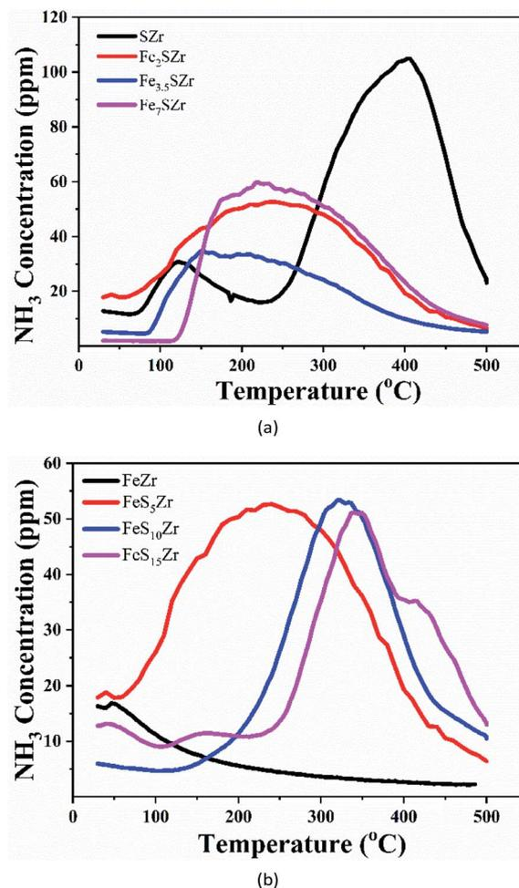
Fig. 5 (a)  $\text{NH}_3$ -TPD of catalysts containing 5%  $\text{SO}_4^{2-}$  and  $x\%$   $\text{Fe}^{3+}$  ( $x = 0, 2, 3.5, 7$ ). (b)  $\text{NH}_3$ -TPD of catalysts containing 3.5%  $\text{Fe}^{3+}$  and  $y\%$   $\text{SO}_4^{2-}$  ( $y = 0, 5, 10, 15$ ).
