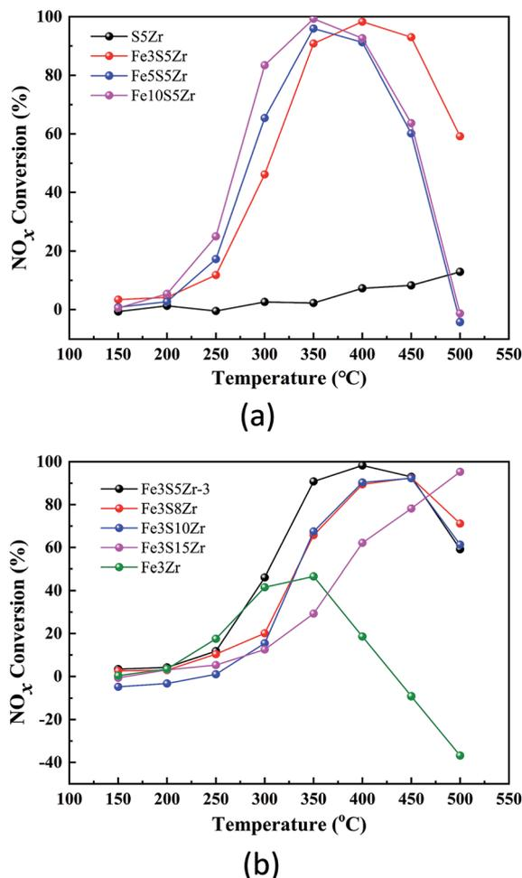
Fig. 1 (a)  $\text{NO}_x$  conversion of catalysts containing 5%  $\text{SO}_4^{2-}$  and  $x\%$   $\text{Fe}^{3+}$  ( $x = 0, 2, 3.5, 7$ ). (b)  $\text{NO}_x$  conversion of catalysts containing 3.5%  $\text{Fe}^{3+}$  and  $y\%$   $\text{SO}_4^{2-}$  ( $y = 0, 5, 10, 15$ ).
