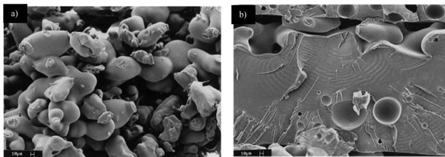
Fig. 12 SLS of PC under (a)  $0.036 \text{ J mm}^{-1}$  and (b)  $0.094 \text{ J mm}^{-1}$  laser density, respectively.<sup>170</sup> Reprinted with permission from Elsevier: *Journal of Materials Processing Technology*, Copyright 1999, License number: 4838261399886.
