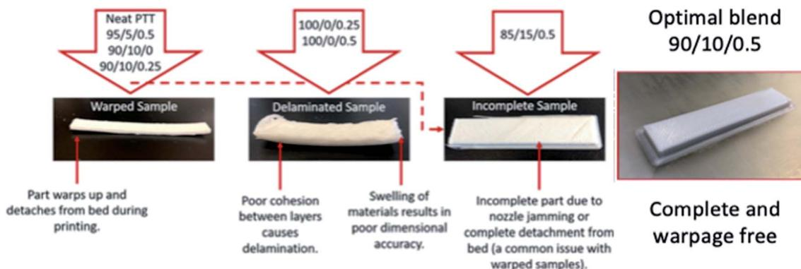
Fig. 8 Optimization of PTT/impact modifier/chain extender blends to make complete samples as novel use for PTT in 3D printing.<sup>6</sup>
