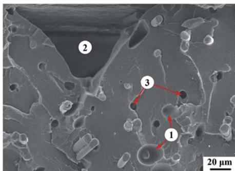
Fig. 16 SEM analysis of the fracture surface of FFF samples.<sup>134</sup> Reprinted with permission from Elsevier: *Composites Part B: Engineering*, Copyright 2019, License: 4694210938408.
