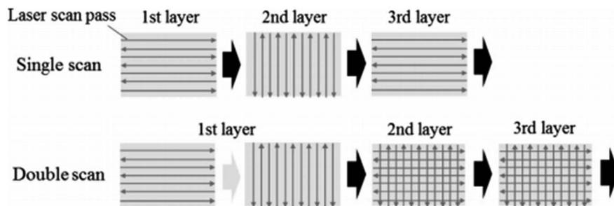
Fig. 9 Single versus double scanning for SLS.<sup>152</sup> Reprinted with permission from Elsevier: *Optics and Laser Technology*, Copyright 2019, License number: 4838260880549.
