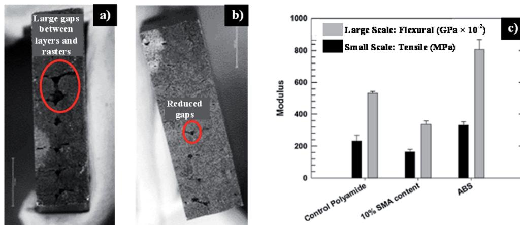
Fig. 14 SEM analysis of the fracture surfaces for BAAM samples (a) PA, (b) PA/ABS compatibilized and (c) a comparison of moduli for small scale versus large scale printing.<sup>7</sup> Reprinted with permission from Elsevier: *Additive Manufacturing*, Copyright 2019, License: 4694241403414.
