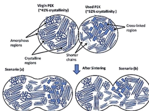
Fig. 11 Two scenarios for re-ordering between virgin and used PEEK powders during SLS.<sup>48</sup> Reprinted with permission from Elsevier: *Journal of Materials Processing Technology*, Copyright 2019, License: 4632510363502.
