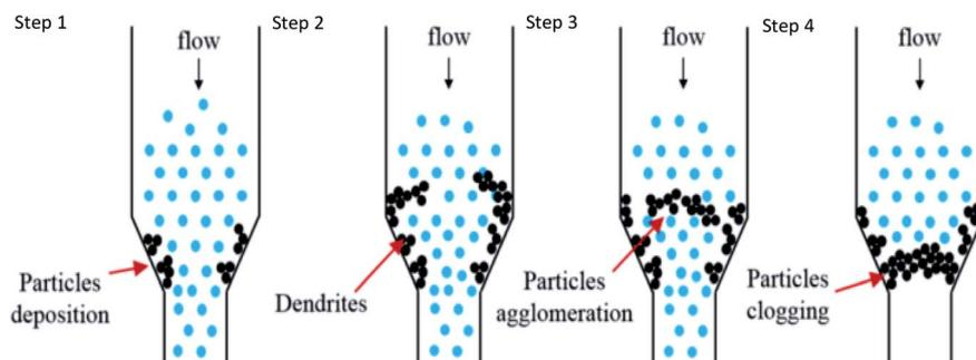
Fig. 13 Modelled clog formation for PC composites *via* FFF.<sup>171</sup> Reprinted with permission from John Wiley and Sons: *Journal of Applied Polymer Science*, Copyright 2019, License: 4732631260702.
