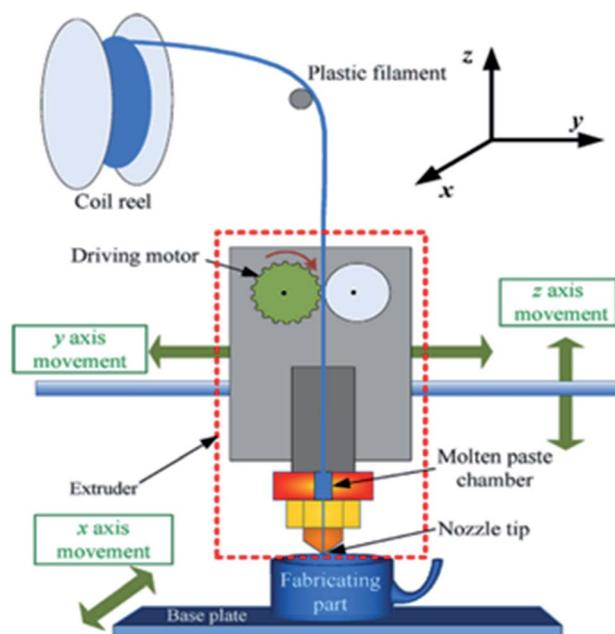
Fig. 2 Schematic representation of fused filament fabrication.<sup>39</sup> Reprinted with permission from Elsevier: *Additive Manufacturing*, Copyright 2020, License: 4743160219820.
