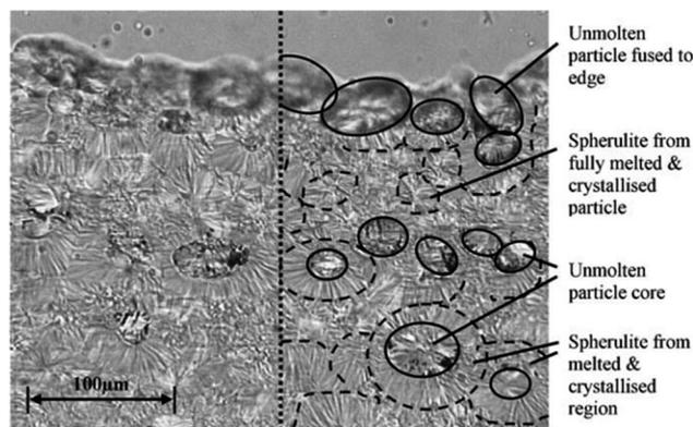
Fig. 6 Optical microscopy image displaying the crystal structure of PA 12.<sup>45</sup> Reprinted with permission from Elsevier: *Materials Science and Engineering: A*, Copyright 2019, License: 4838261169022.
