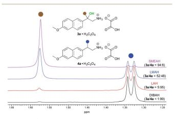
Fig. 2 Partial  $^1$ H NMR (400 MHz, DMSO- $d_6$ , 35  $^{\circ}$ C) spectra showing the 3a/4a ratio affected by the type of the complex metal hydride.
