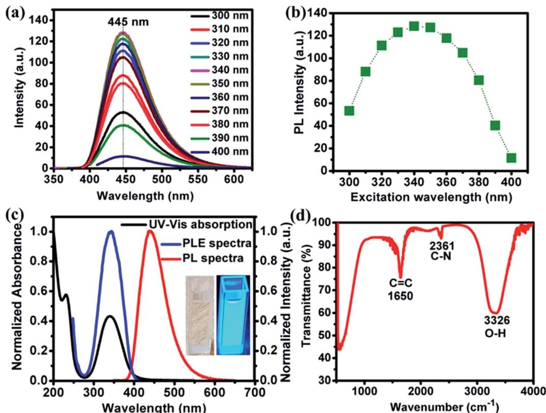
Fig. 1 (a) PL emission spectra of NOCDs at different excitation wavelengths, (b) variation of PL peak emission intensity at 445 nm as a function of different excitation wavelengths (maximas from (a) vs. excitation wavelength), (c) UV-vis absorption, PLE (corresponding to emission at 440 nm) and PL emission spectrum (excited at 340 nm); inset images are photographs of NOCDs in normal daylight and under 365 nm UV irradiation (d) FTIR spectrum corresponding to as prepared NOCDs.
