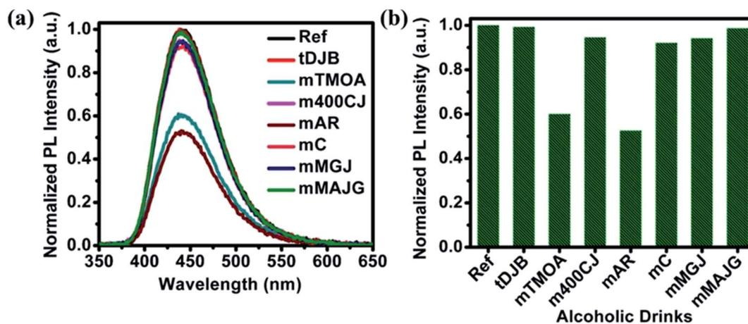
Fig. 5 Fluorescence response of NOCDs in the presence of diluted unspiked branded and unbranded alcoholic beverages (a) normalized PL emission measured at  $\lambda_{\text{ex}} = 340 \text{ nm}$  (b) bar diagram representing the PL peak emission from NOCDs.
