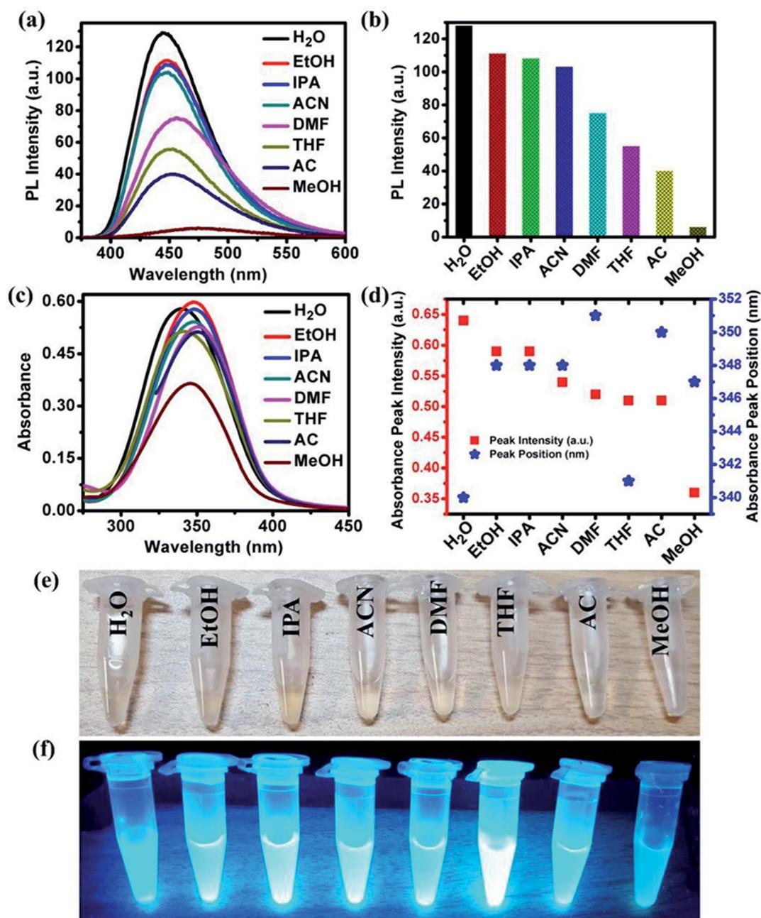
Fig. 2 Fluorescence of NOCDs in different solvents (a) PL spectra ( $\lambda_{\text{ex}} = 340$  nm) (b) variation in PL peak intensity (taken from (a)), (c) UV-vis absorption spectra, (d) peak absorption of NOCDs in different solvents, (e) photographs of NOCDs in different solvents under daylight and (f) NOCDs in different solvents irradiated by UV lamp ( $\lambda_{\text{ex}} = 365$  nm).
