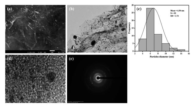
Fig. 2 (a) FESEM image of Pt-Ag/Gr. (b) TEM image of Pt-Ag/Gr. (c) The particle size distribution histogram of Pt-Ag. (d) HRTEM image of Pt-Ag/ Gr. (e) SAED pattern of Pt-Ag.
