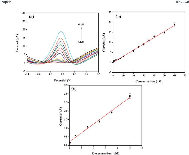
Fig. 6 (a) Differential pulse voltammograms with various DA concentrations (0.1, 1, 3, 5, 7 10, 20, 25, 30, 35, 40, 50, 60 μΜ) at Pt-Ag/Gr/GCE in 0.1 mol L<sup>-1</sup> PBS at pH 6.5. (b) Relationship between peak current and DA concentration. (c) The calibration curve in low concentration range.
