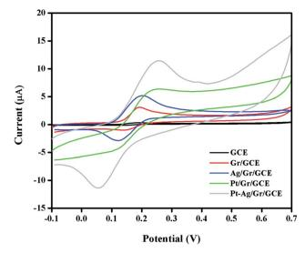
Fig. 5 Cyclic voltammograms of 25  $\mu$ M DA in 0.1 mol L<sup>-1</sup> PBS (pH 6.5) at a scan rate of 20 mV s<sup>-1</sup> on bare GCE, Gr/GCE, Ag/Gr/GCE, Pt/Gr/GCE and Pt-Ag/Gr/GCE.
