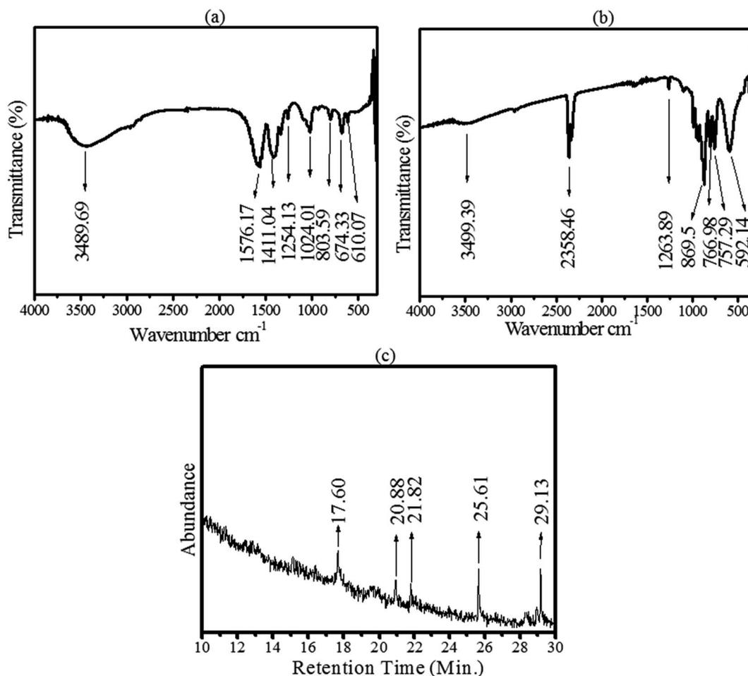
Fig. 2 Identification of organic stabilizing agents of  $\text{CoMoO}_4$ . (a) FTIR spectra of  $\text{CoMoO}_4$  after drying at 95 °C. (b) FTIR of  $\text{CoMoO}_4$  after annealing at 450 °C, and (c) GC-MS spectra of  $\text{CoMoO}_4$ .
