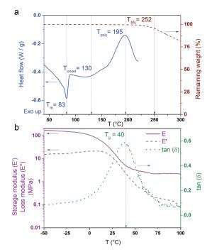
Fig. 2 (a) DSC thermogram (N<sub>2</sub>, 10 °C min<sup>-1</sup>) of CAR-4apds overlapped with TGA (N<sub>2</sub>, 10 °C min<sup>-1</sup>). (b) DMTA thermogram of poly(CAR-4apds). Storage modulus (E'): solid line, loss modulus (E''): dashed line and tan  $(\delta)$ : dotted line.
