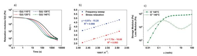
Fig. 3 (a) Stress relaxation curves for poly(CAR-4apds) between 110 °C and 140 °C. (b) Arrhenius plots obtained from stress relaxation values where  $G/G_0 = 1/e$  and from G' and G'' crossover from frequency sweep tests, with fitting curves. (c) Frequency sweep curves for poly(CAR-4apds) at 140 °C.
