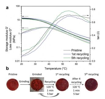
Fig. 5 (a) Dynamic mechanical thermal analyses of the pristine poly (CAR-4apds) and after the first and fifth reprocessing. (b) Reprocessing procedure to obtain discs.
