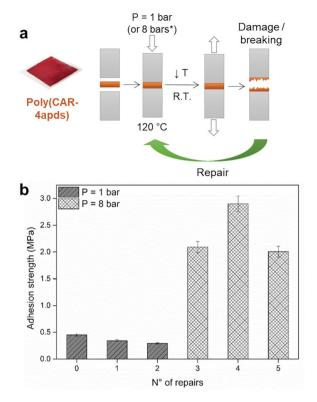
Fig. 6 Reversible and self-healing adhesive with the poly(CAR-4apds) membrane. (a) Illustration of the fabrication film from poly(CAR-4apds) and schematic representation of the adhesion test procedure. (b) Adhesive strength of the pristine sample and after 5 repair cycles.
