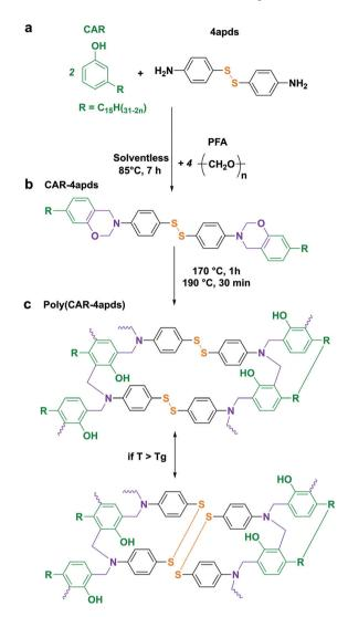
**Scheme 1** Chemical structure of the disulfide-benzoxazine vitrimer. (a) Synthetic route of CAR-4apds (*n* can be 0, 1, 2 or 3). (b) Schematic representation of the CAR-4apds monomer and polymerization conditions. (c) Simplified cross-linked network and mechanism of chemical bond re-arrangement upon heating showing the dynamic properties of poly (CAR-4apds).
