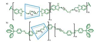
Fig. 29 (a) Yamaguchi, Osakada and Yamamoto's benzimidazole-based poly[n]rotaxane, and (b) Simionescu's imine poly[n]rotaxane.
