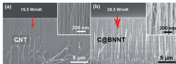
Fig. 13 Scanning electron microscopy (SEM) images of (a) VA-CNTs and (b) VA-MWCNTs coated in h-BN. The h-BN coating increased thermal conductivity of the aligned assembly from 15.5 W m<sup>-1</sup> K<sup>-1</sup> to 29.5 W m<sup>-1</sup> K<sup>-1</sup>. Reproduced with permission from ref. 22. Copyright 2017, American Chemical Society.
