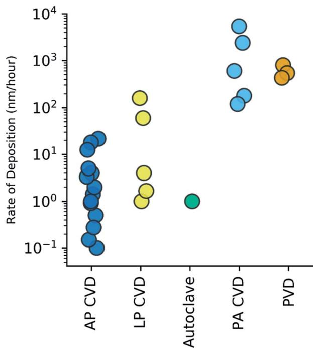
Fig. 5 Calculated h-BN deposition rate (nm per hour) amongst the various methods of CVD (atmospheric pressure,<sup>21,27–35</sup> low pressure,<sup>20,36–38</sup> autoclave,<sup>39</sup> plasma assisted<sup>40,41</sup>) and PVD.<sup>41</sup> Rates are shown on a log 10 scale.
