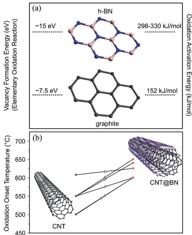
Fig. 11 (a) Vacancy formation energy<sup>78,83</sup> and oxidation activation energy<sup>52</sup> of h-BN vs. graphitic carbon, justifying why h-BN is more oxidatively stable at high temperatures than graphitic carbon. (b) Compiled oxidation onset temperature values from studies that reported TGA results on CNTs prior to h-BN coating and after h-BN coating,<sup>21,27,30,31,39,50</sup> suggesting that h-BN was effective at improving oxidation resistance.
