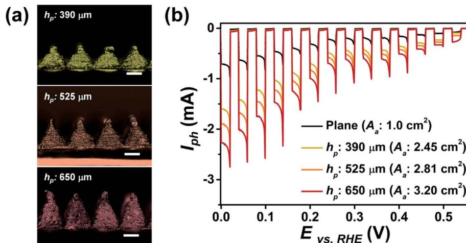
Fig. 4 (a) Optical images of the fabricated 3D photoelectrodes composed of 400 pyramids. The total light absorption area ( $A_a$ ) of the 3D photoelectrodes is modulated by adjusting  $h_p$  to 390, 525, and 650  $\mu\text{m}$  (fixed  $L_b$ : 490  $\mu\text{m}$ ). The scale bar is 250  $\mu\text{m}$ . (b) Chopped-light PEC performance of the p–n homojunction  $\text{Cu}_2\text{O}$  electrodes with planar and 3D pyramid shapes with respect to the total light absorption area ( $A_a$ ).
