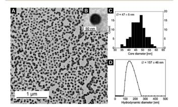
Fig. 2 (A) TEM image of sample 4, the cores of the micelles with the embedded [Zn(OAc)<sub>2</sub>(bipy)]<sub>n</sub> CP nanoparticles appear black, (B) an inset with a zoom on a single nanoparticle, (C) core size distribution  $D_{\text{core}}$  (from TEM) and (D) hydrodynamic diameter distribution  $D_{\text{h}}$  (from DLS) of the nanocomposite sample 4 (for DLS autocorrelation function see Fig. S6†).
