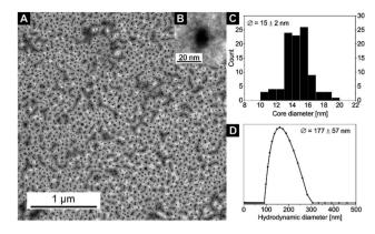
Fig. 4 (A) TEM image of sample 7. (B) An inset with a zoom on a single nanoparticle. (C) Core size distribution  $D_{core}$  (from TEM) and (D) hydrodynamic diameter distribution  $D_h$  (from DLS) of nanocomposite sample 7 (for DLS autocorrelation function see Fig. S11†).
