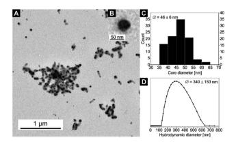
Fig. 5 (A) TEM image of sample 8. (B) An inset with a zoom on a single nanoparticle. (C) Core size distribution  $D_{core}$  (from TEM) and (D) hydrodynamic diameter distribution  $D_h$  (from DLS) of sample 8 (for DLS autocorrelation function see Fig. S11†).
