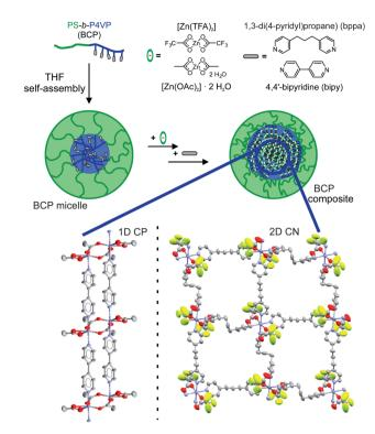
Scheme 1 Synthetic approach for the preparation of Zn-based CP-BCP nanocomposites. An excerpt of the crystal structures of both CP bulk materials is given below (left:  $[Zn(OAc)_2(bipy)]_n$ , right:  $[Zn(TFA)_2(bppa)_2]_n$ ).
