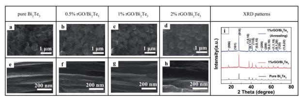
Fig. 1 Surface and cross-sectional SEM images of  $Bi_2Te_3$  nanoplate films with different mass ratio of rGO nanosheets: (a) and (e) pure  $Bi_2Te_3$ , (b) and (f) 0.5% rGO/Bi<sub>2</sub>Te<sub>3</sub>, (c) and (g) 1% rGO/Bi<sub>2</sub>Te<sub>3</sub>, and (d) and (h) 2% rGO/Bi<sub>2</sub>Te<sub>3</sub>; (i) XRD patterns of the pure Bi<sub>2</sub>Te<sub>3</sub> and 1% rGO/Bi<sub>2</sub>Te<sub>3</sub>, composites films before and after annealing
