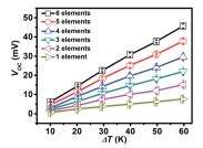
Fig. 4 Open circuit voltage ( $\Delta V_{oc}$ ) against temperature difference ( $\Delta T$ ) responsible for number of thermal elements of flexible TEG devices made from pure Bi<sub>2</sub>Te<sub>3</sub> nanoplates. Error bars are estimated from repeatability of the experimental results: for each material-making condition, three samples are prepared and measured.
