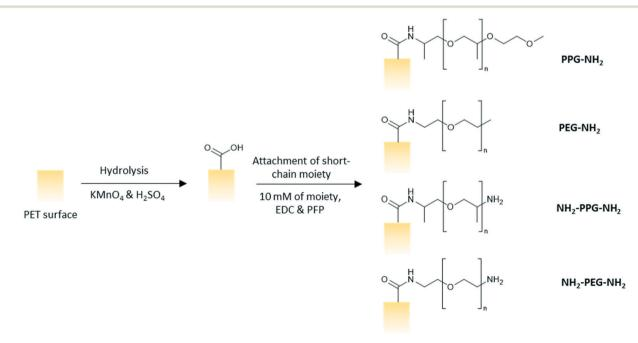
Fig. 2 Schematic of modification process on either a PET coated silicon wafer or on a PET membrane surface (note: possible partial charges are not shown).
