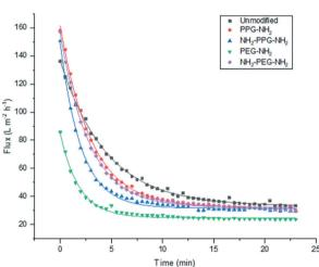
Fig. 6 Comparison of (a) adsorbed mass of lysozyme before and after forward flushing with PBS and (b) recorded flux during fouling tests. Trendlines were added to guide the eye.
