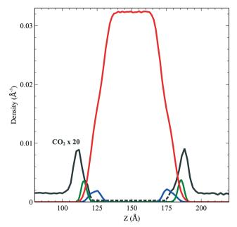
Fig. 5 Density profile of C<sub>12</sub>E<sub>6</sub> (head with blue lines and tail in green) and water (red) with the probability to find CO2 (dark line).
