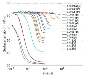
Fig. 8 Dynamic surface tensions of clean surface adsorption in C<sub>12</sub>E<sub>6</sub> aqueous solution at different concentrations.
