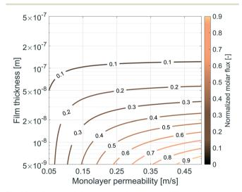
Fig. 14 Influence of the gas monolayer permeability and water core thickness on the dimensionless molar flux. The diffusive flux was normalized by the maximum flux, equal to  $9.303 \times 10^{-5} \text{ mol m}^{-2} \text{ s}^{-1}$ , obtained with the maximum value of  $k_{\rm ML} = 0.5~{\rm m~s^{-1}}$  and for the minimum value of  $h = 5 \times 10^{-9}$  m.
