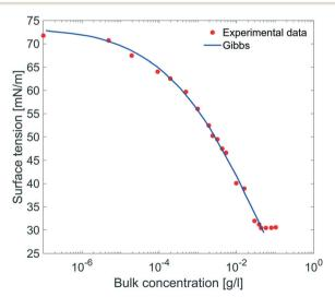
Fig. 9 Equilibrium surface tension from Fig. 8 as a function of bulk concentration and compared with the results obtained using the Gibbs adsorption egn (4)
