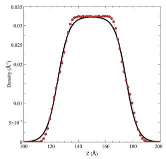
Fig. 3 The water density profile was fitted to the function presented in eqn (2). With it, an average Gibbs dividing interface is defined at  $\rho = \frac{1}{2}(\rho_{\rm L} + \rho_{\rm V})$ . Also the hydration layer is estimated from the fitted d.
