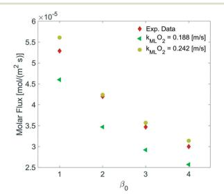
Fig. 11 Dependence of the molar flux of oxygen on the permeability for a film thickness of 5 nm against experimental data from ref. 5.
