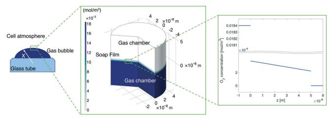
Fig. 10 Left-hand side: A sketch of the shrinking bubble in the Princen<sup>38</sup> experimental setup. Middle: Continuum model results for oxygen diffusion through the soap film. Right-hand side: O2 concentration distribution across the soap film.
