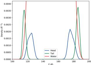
Fig. 2 Mass density profile. The red curve corresponds to the water density. The surfactant density was separated into the hydrophobic tail and hydrophilic head. From the figure, the permeation of the water onto the hydrophobic region is shown. Also, the width of the tail/head layer of the surfactant is computed and presented in Table 1 using eqn (3).
